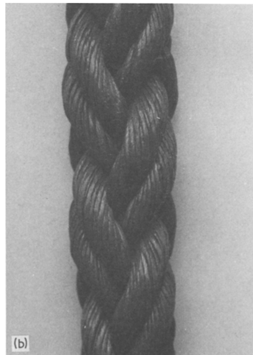
Figure 7 Man-made fibre ropes (a) double-braided, and (b) eight-strand plaited (courtesy of Bridon Fibres and Plastics Ltd).
